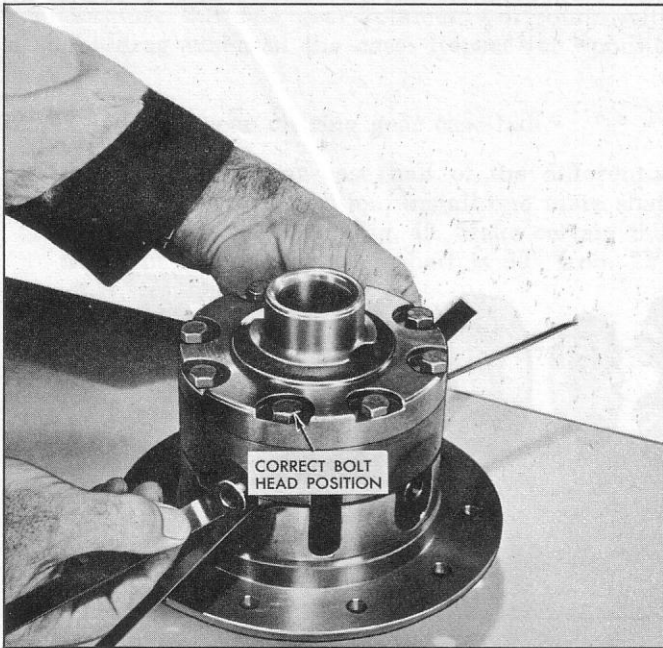
Fig. 34—Checking Shaft and Ramp Clearance
