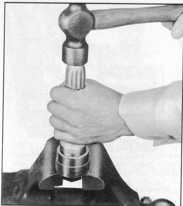
Fig. 16—Installing Mainshaft Bearing Cup
